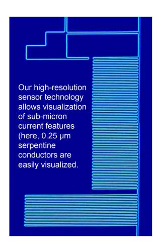
Micro Magnetics now offers CS1000 imaging on a contractual per-hour basis. Our non-invasive magnetic imaging requires no sample preparation and allows you to see the flow of current on all levels of your sample, overlaid over crisp high-resolution optical images of the device. Our software and analysis capabilities allow us to determine the strength and depth of current flow, which enhances the localization capabilities and also allows us to validate new designs.
