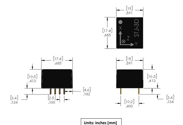
STJ-3D: Positions of Magnetic Sensors for X-Axis, Y-Axis, and Z-Axis
