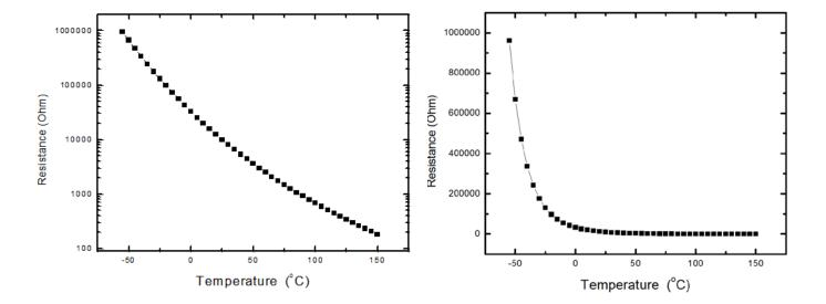
To determine the temperature (T in the units of Celsius °C), measure the resistance (R in the units of Ohm) of the thermistor. Then calculate the temperature using the following formula,
